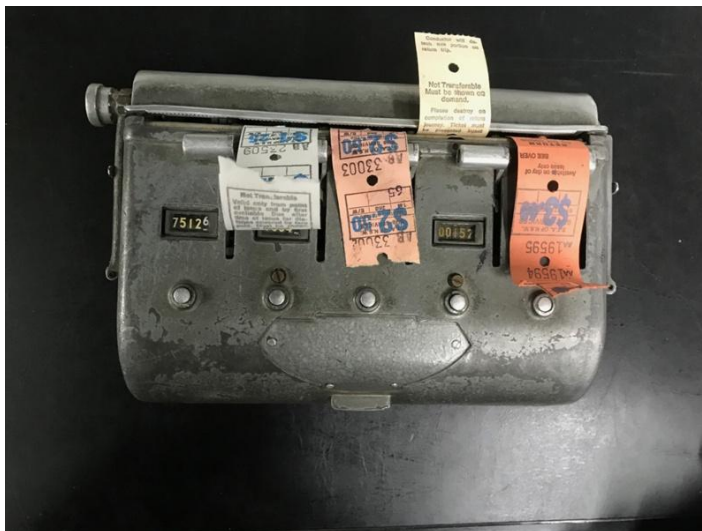
Bell Punch Ultimate Ticket Machine GT187, manufactured London, 1949, Sydney Bus Museum collection.
