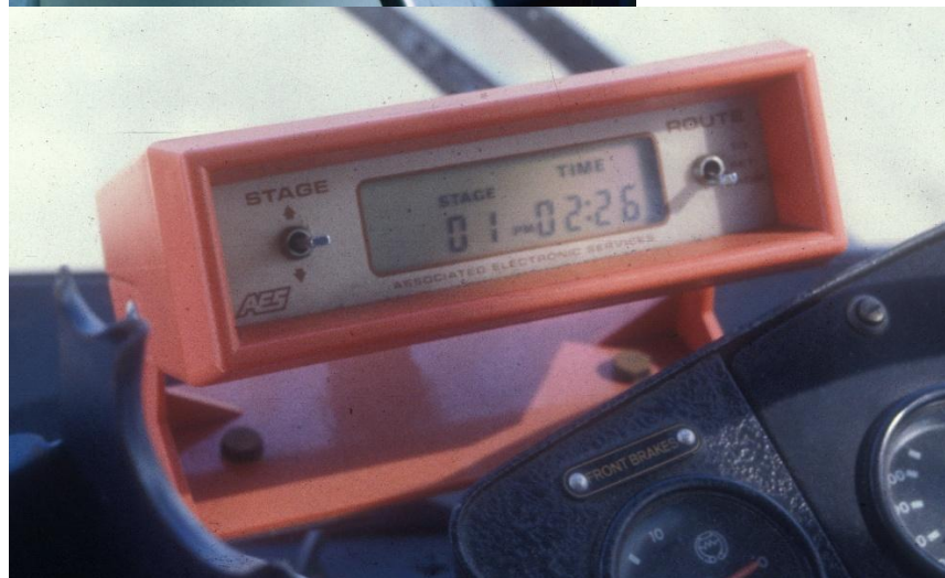
AES MetroTen remote control unit showing section number and time. Greg Travers
